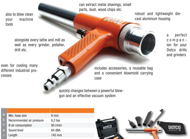
Weight0,68 kgAir inlet thread1/4" NPTVibration (m/s²)< 0,4 m/s²</td>
